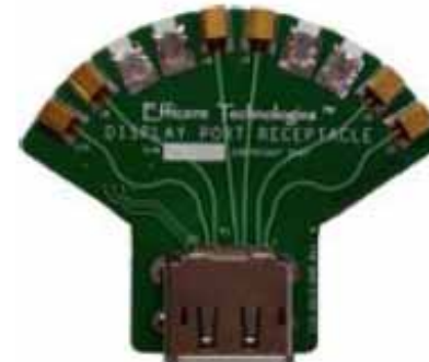
DisplayPort receptacle and Receptacle Calibration boards. (not to scale)
